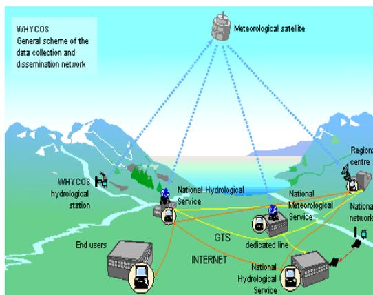
Figure 7: Satellite DCP Operation
