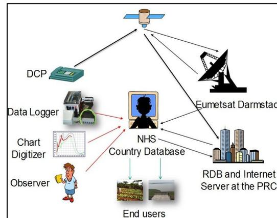
Figure 8: Satellite DCP Operation
