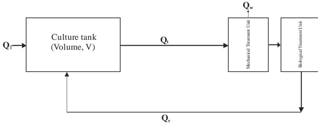
Figure 1: Schematic Diagram of a Recirculating Aquacultural System
